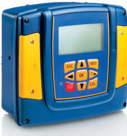
The DULCOMETER® diaLog DACa multi-parameter controller is the new controller platform from ProMinent. It replaces the D1Ca/D2Ca controllers. The diaLog DACa can also be installed in a control cabinet using the optional mounting kit. The diaLog DACa has been specifically developed for the continuous control of liquid analysis parameters in water treatment processes, environmental technology and industry.
