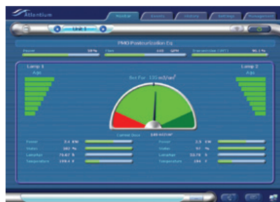
The monitor displays the status of real-time data, including actual dose delivered
