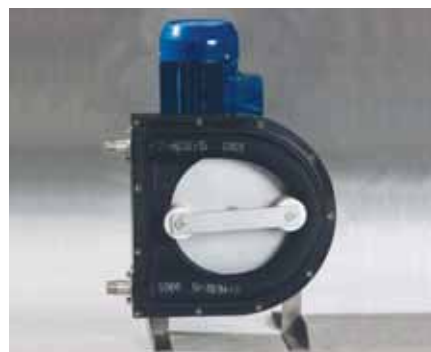
Model LSM-010 without the cover. The hose and fittings are the ONLY wetted part. The soft rollers, unique adjustment system and larger diameter ensure longer hose life and lower operating costs.
