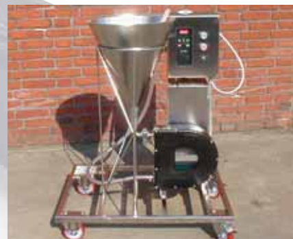
Special LSM-010 dosing unit for injection of jam into ice cream (Ghana, Africa). This design will handle many similar dosing applications, and is available tailor made for your applications.
